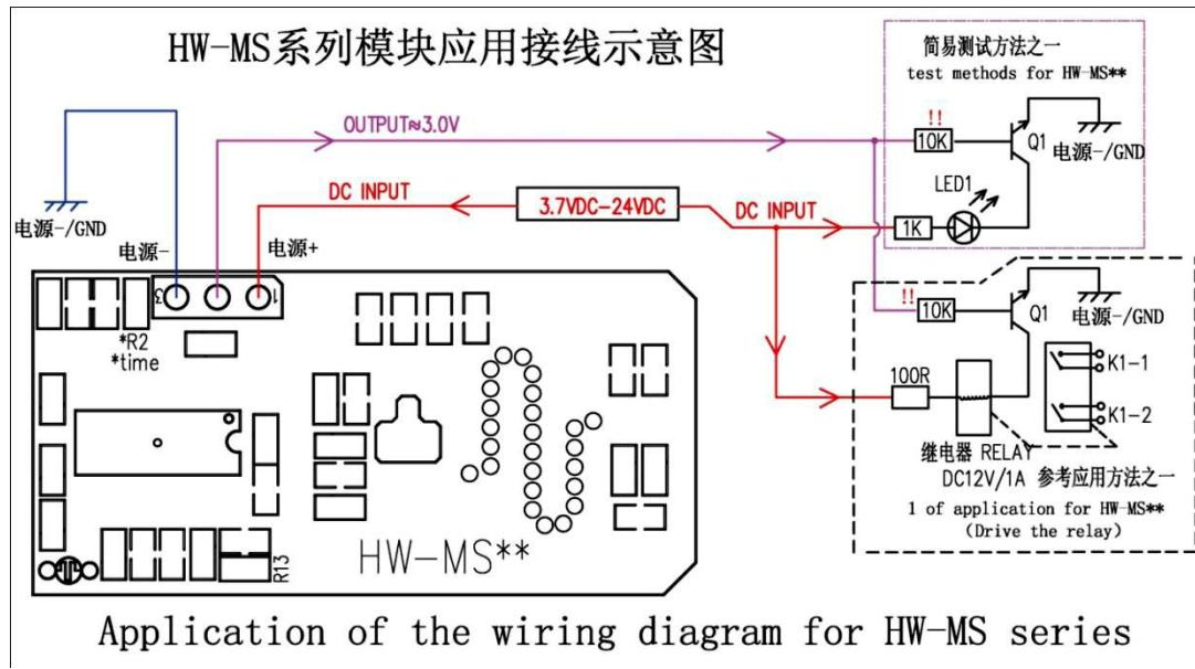
Application of the wiring diagram for HW-MS series
